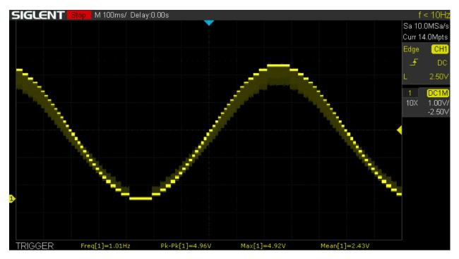
Noise comes from USB traffic and it is in kHz region. Since ADC output frequency is much lower, it can be greatly reduced with a simple RC low pass filter.
