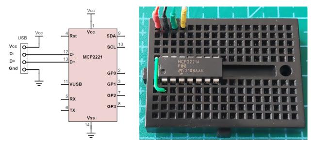
Although this is **not a recommended design**, it should work fine. See the MCP2221 data sheet for more information. Import EasyMCP2221 module and try to create a new *Device* object with default parameters.
