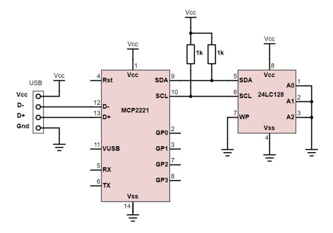
This is it in the breadboard. Don't forget to connect WP pin to either Vcc or Gnd.
