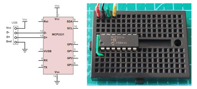
Although this is **not a recommended design**, it should work fine. See the MCP2221 data sheet for more information. Import EasyMCP2221 module and try to create a new *Device* object with default parameters.
